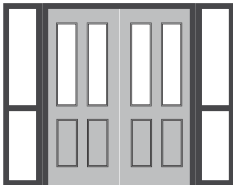
Double Doors with Glazed Sidelights and Midrails
